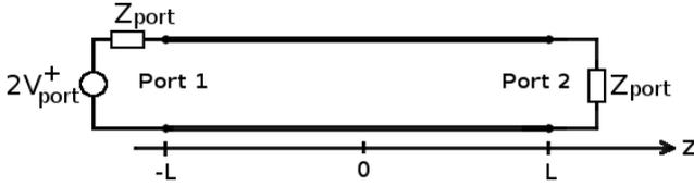
**Fig. 9:** Simulation setup for obtaining  $2 \times 2$  S matrices for different TL lengths.
