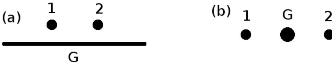
FIG. 2: Cross sections examples of two conductors having the same geometry relative to ground: a. two wires above an “infinite” ground plane, and b. two wires symmetric around a ground wire.
