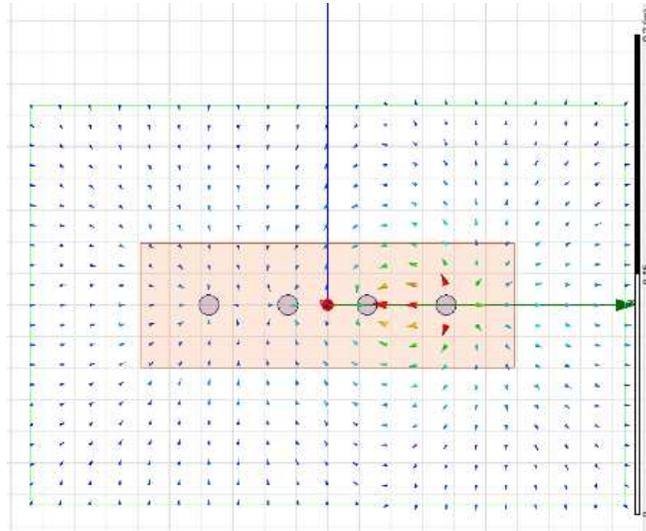
FIG. 5: Cross section of the conductors inside the insulator. The arrows show the electric field for some feeding and one remarks that it is partially in the insulator and partially in the surrounding space. We used the relative dielectric constant  $\epsilon_r = 2.1$ . We simulated the cases of  $\tan \delta$  equal 0 or 0.001 and the cases of copper or ideal conductors.
